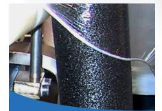
**Pallet Grip** *rolls* the bottom 5 inches of the stretch film web into a tight film cable during the last seconds of the wrap cycle.
