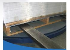
The cable is placed (*driven down*) just below the top boards of the pallet, low enough to lock the load yet high enough to avoid the forks from pallet jacks or lift trucks.
