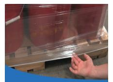
**Pallet Grip** *locks* the *load* to the pallet with a film cable.
