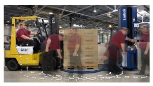
S-300XT automatically attaches and cuts the film. Equipped with a fully protected mechanical cut & clamp. Improve productivity by keeping the operator on the forklift.
